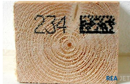
Marking of Wooden Beams
